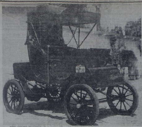
THE NIGHT CLOSING of gasoline filling stations doesn't worry the driver of this 1935 Popo-Waverly as the illuminated car is driven by an electric motor, George G. Cannon, the owner, located the car in the dark.
