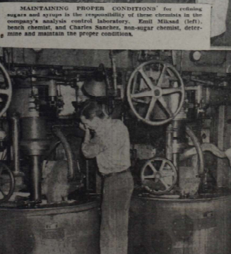
THESE CENTRIFUGALS WHIP MOLASSES OFF THE SUGAR. A spin dry device like those in some washing machines, this high-speed perforated drum removes the syrup from a sugar and syrup mixture and purges the retained sugar crystal which emerges white.
