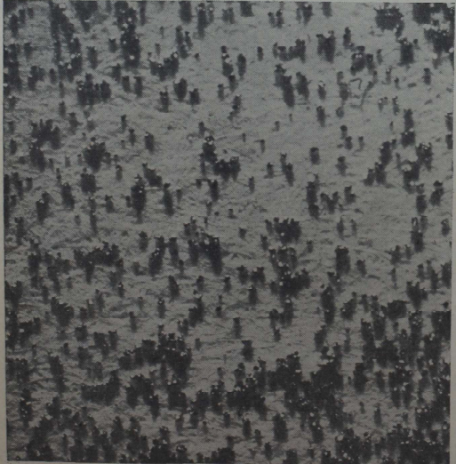
DON'T BELIEVE your eyes! This isn't Coney Island on an August Sunday. Enlarged 23 times, the picture shows the action of corrosion by sulphuric acid, copper sulphate and water on stainless steel.
