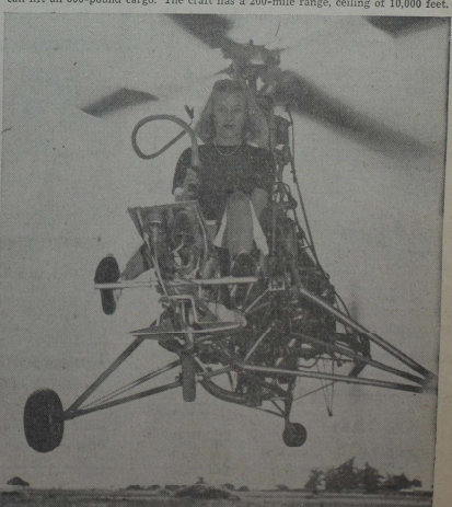
ON HER OWN, Winnie is soloing despite a 20-mile wind that buffers craft. The rotor heads of other helicopters have several hundred parts. This one has seven.
