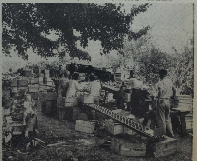
AUTOMATIC SORTING is employed at Outhouse Orchards to grade and polish apples for the market. The fresh picked fruit is poured into one end of the machine and graded to size while working its way between two revolving soft-cushioned cylinders
